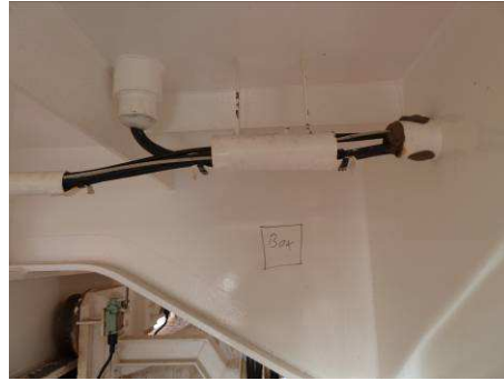
Antenna cable and air pipe, outside the funnel, under the wing
