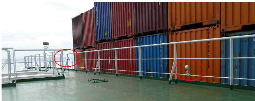
Inmarsat-C and GPS antenna on the wing, portside.
