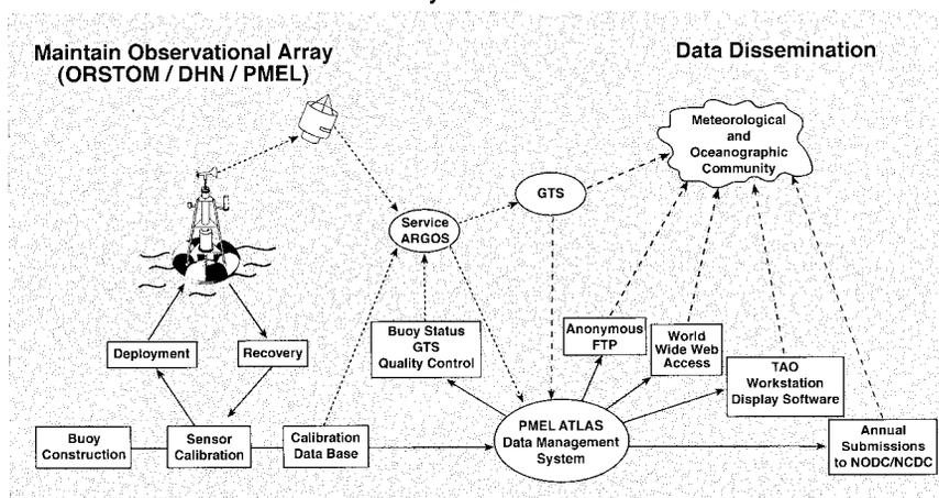
FIG. 7. Schematic of the PIRATA real-time data flow.
